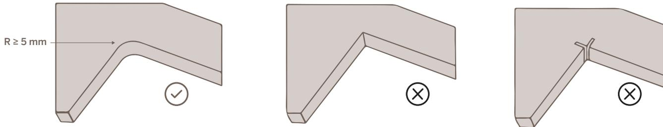
Although not advised, 90° internal angles may be obtained using a water-jet process. This finish increases the possibility of cracking during processing, handling, transport and installation of the top, and the subsequent settling of the various kitchen units.
