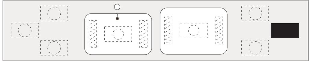
The correct positioning of the suction cups supporting the slab is a fundamental aspect for successful cutting. For this reason, distribute the suction cups evenly to support the slab particularly near the cut and below the part to be removed after cutting.
