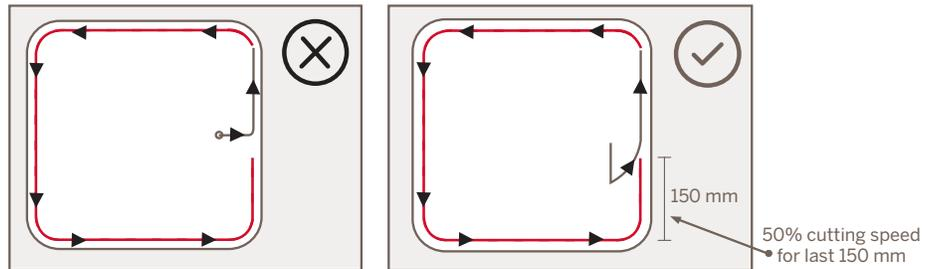
With the cutting feed, it is important to avoid any bending/binding between the part to be removed and the part machined as this may cause cracks and/or breakages. As an alternative to the suction cups, special clamps can be used: in this case, bear in mind that the part the clamp is positioned on cannot be machined.
