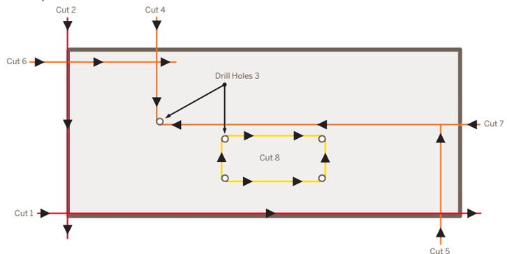
Crossville Porcelain Slabs can be machined with numeric control machinery (CNC).
