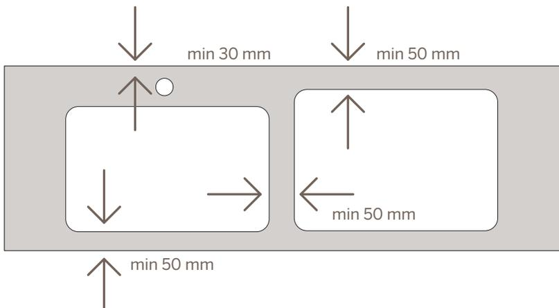
In the design of a kitchen top, maintain a minimum distance of 50 mm (2 in) from the outer edge with large holes and grooves. The same minimum distance must be maintained between adjacent openings.
