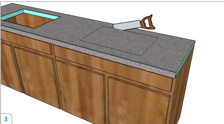
3 Cut out for the sink using a jigsaw or handsaw. As needed, recess cuts might be created with a utility knife or a router to accommodate recessed sinks. Cutting the holes may proceed before or after installation of Laminam as indicated in step 5.
