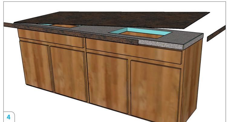
4 Install the Laminam over the wedi Building Panel surface and edges using a modified thinset according to section 7.1 of the Laminam Technical Manual/ Guidelines found at: <http://laminambycrossville.com/TechnicalGuides.html>
